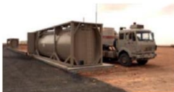
THIELMANN WEW Transportable Fuel Station In service in the Middle Ea
